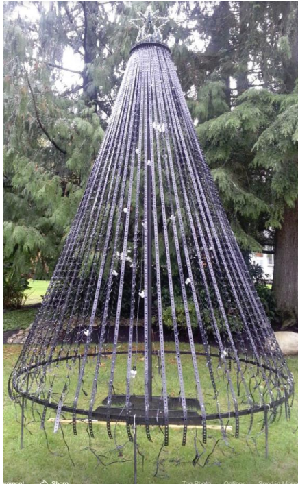
RGB/Pixel Tree 15ft - 270 Degree 15 Universes 56 50ct strips, 2800 nodes 2 Advatek controllers & nodes
