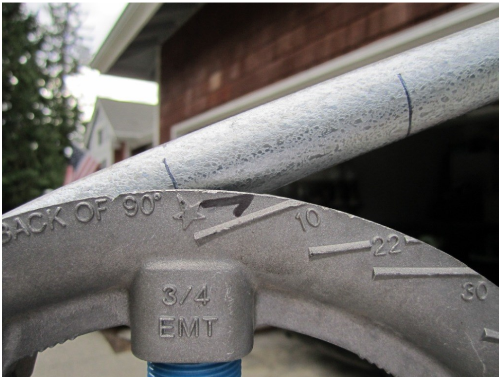
Picture 11 - 5 degree & EMT Relationship After Pull
