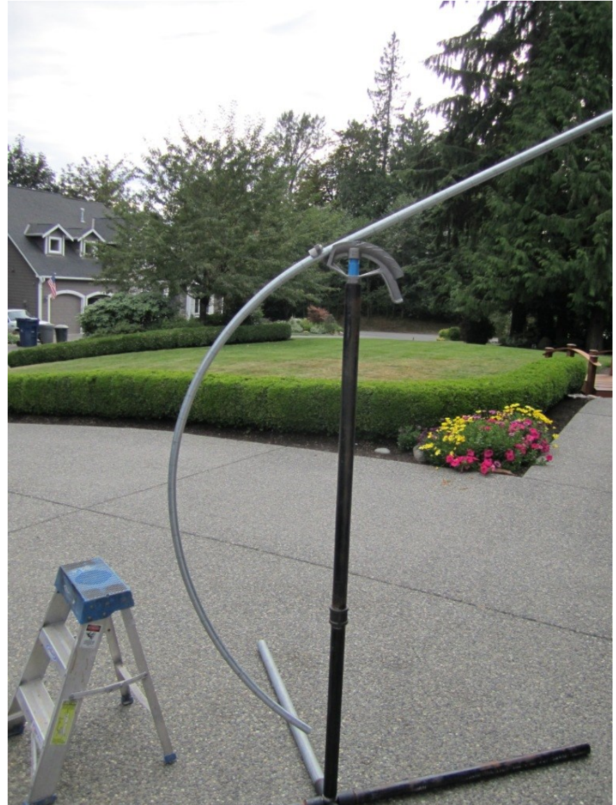
Picture 8 - EMT Inserted Into Bender
